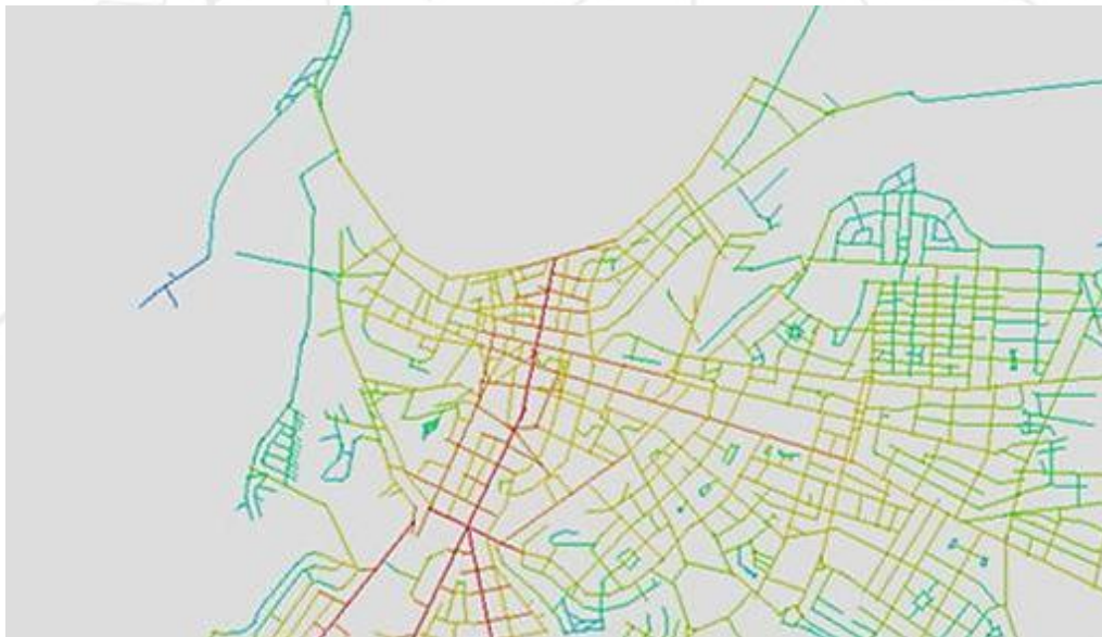
FIG 87: INTEGRATION ANALYSIS ON THE UNALTERED ROAD NETWORK AXIAL MAP 2008 DEPTHMAPX 0.8.0. SOURCE: AUTHOR
